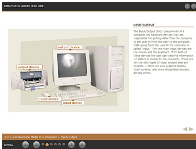
Figure 1: A screen shot explaining input and output devices of a computer.
